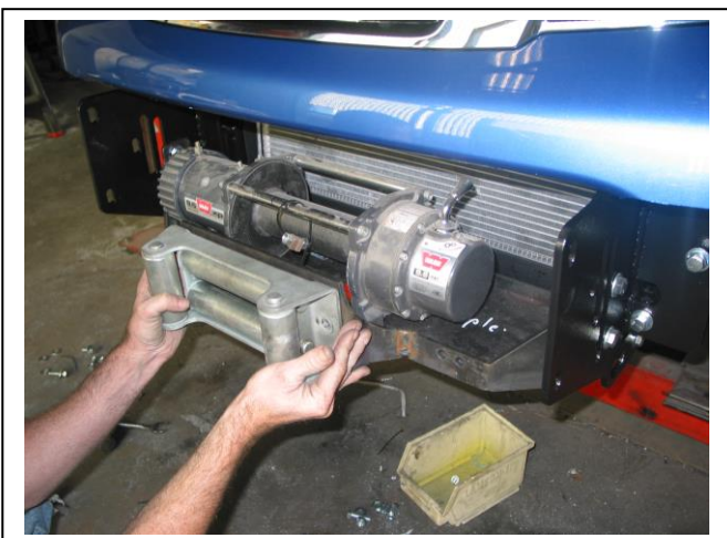
Figure 5: Fairlead rollers being attached to winch frame
