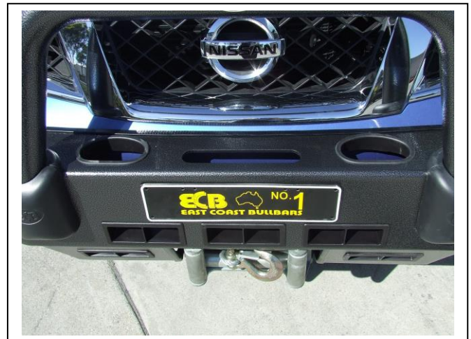
Figure 16: Inspection holes in top of Protection Bar
