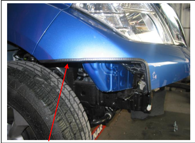
Figure 13: 3mm clip lock trim on outer cut edge of plastic bumper.
