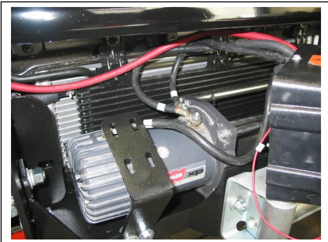
Figure 7: Ensure winch wiring is clear of hot and sharp objects.
